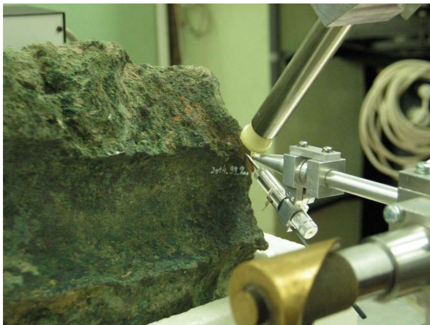
Figure 2. A gun fragment bombarded with external proton beam of 3 MeV energy for PIXE analysis.
